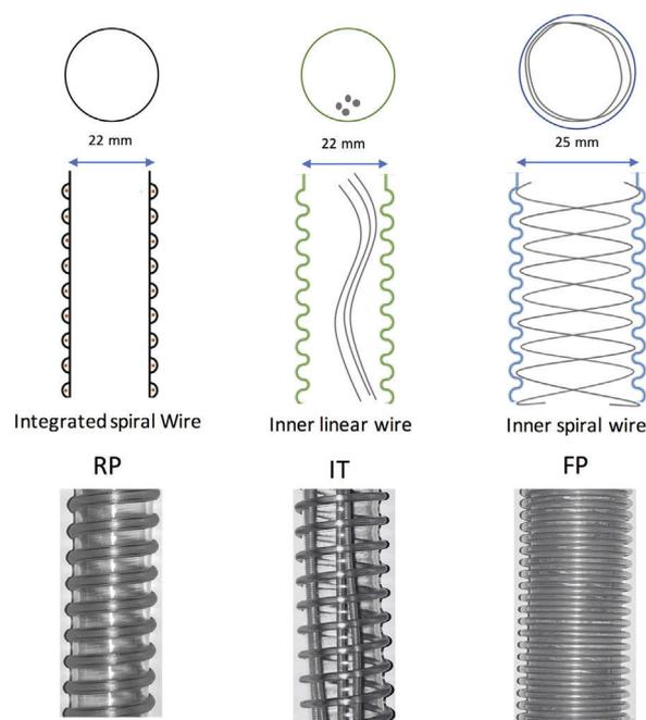
Fig. 1. Heated wired-circuits.
