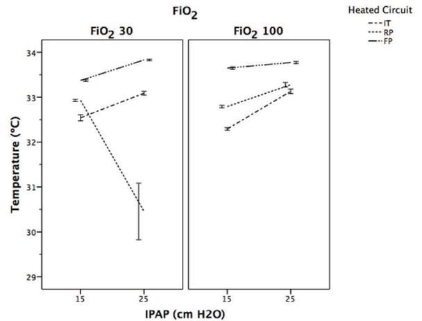
Fig. 6. Evolution of temperature ( $T$ ) following a change in IPAP levels at different FiO<sub>2</sub>. Data expressed as means and CI 95%.  $P < .001$  for each FiO<sub>2</sub> study group between different IPAP levels. Key: FP= Fisher & Paykel RT-319; RP= Respironics 1045770; IT= Intersurgical B/SYS 5809001.
