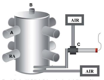
Figure 1. Chamber. A) Individual cylinders to place the animals. B) Output of cigarette smoke. C) Venturi valve.
