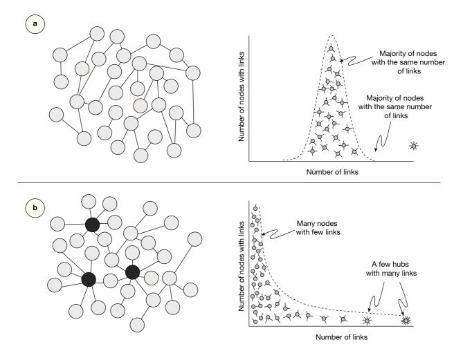
**Figure 2.** Examples of networks with Poisson topology (*a*) and scale-free topology (*b*). In each case, the relationship between the number of nodes with links and the number of links (x axis) is shown.
