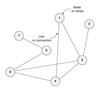
**Figure 1.** Schematic representation of a network with 7 nodes and 8 links. The set of nodes is  $P = \{1, 2, 3, 4, 5, 6, 7\}$ , and the set of links is  $E = \{\{1,3\}, \{1,4\}, \{2,3\}, \{3,4\}, \{3,6\}, \{4,6\}, \{6,5\}, \{5,7\}\}$ .
