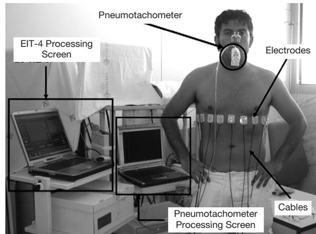
Figure 1. Arrangement of 2 units. On the right, the electrodes around the chest. The pneumotachometer is connected to the volunteer's mouth. On the left, the computer equipment used for the study. Both tests were controlled with a laptop computer. EIT indicates electrical impedance tomography.
