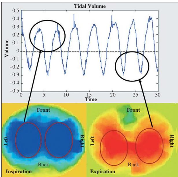
Figure 2. The lower panel shows electrical impedance tomography image obtained during maximum inspiration and expiration for calculating tidal volume, shown in the top panel.
