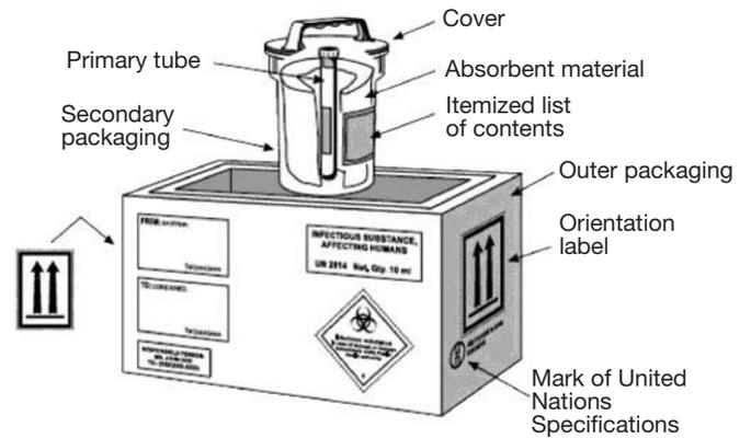
**Figure 3.** Schematic representation of UN 2814 packaging. (Diagram taken from the World Health Organization Guidelines on the transport of infectious substances, 2007-2008.<sup>49</sup>)
