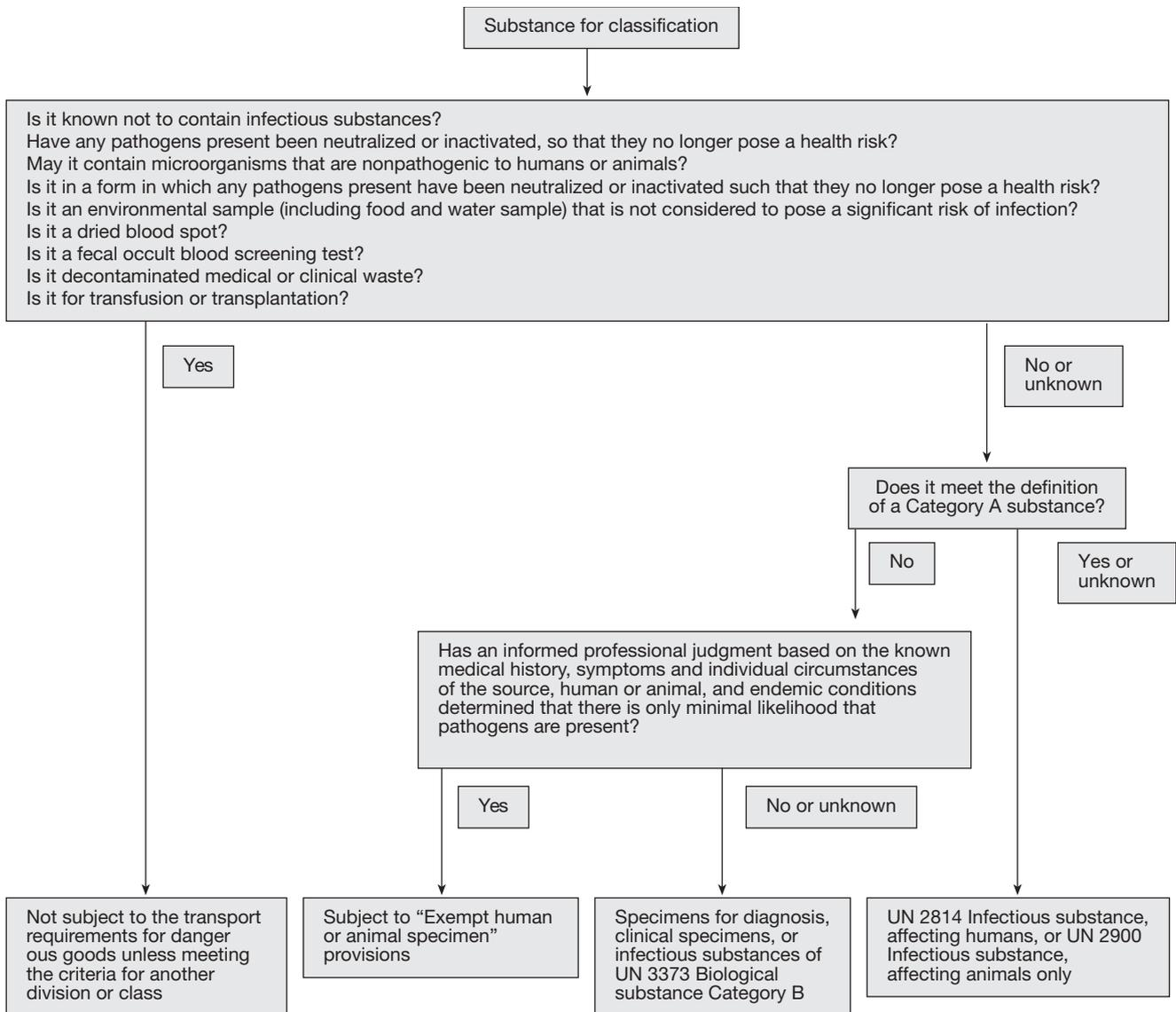
**Figure 1.** Flowchart for classifying biological specimens according to the UN classification. (Diagram taken from the World Health Organization *Guidelines on the transport of infectious substances, 2007-2008*.<sup>49</sup>)
