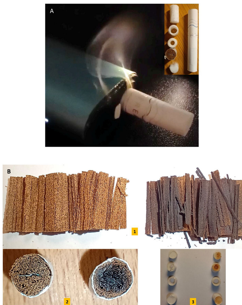
Fig. 1. (A) Smoke delivered by unit, and exploded view of a specific cigarette for induction use. (B) Changes in tobacco and filters. For all images: on the left before, on the right after smoking. Note the charring of the tobacco, (1) Tobacco extracted from the specific cigarette of the device. (2) Device-specific cigarette modified tobacco plug (note the inductive metal located in direct contact with the tobacco). (3) Filters normally in the body of the cigarette.
