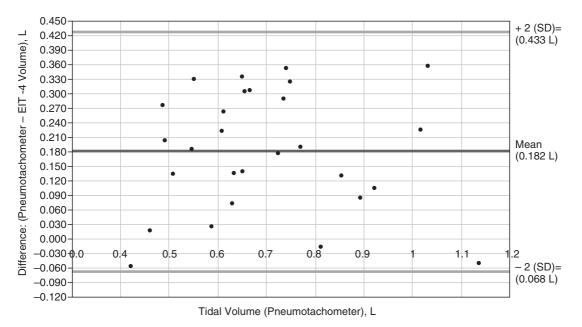
Figure. Band-Altman Plot. Distribution of tidal volume measurements with respect to pneumotachometer values. EIT, electrical impedance tomography; SD, standard deviation.
