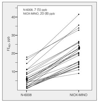
Figure 2. Comparison of fraction of exhaled nitric oxide (FE<sub>NO</sub>) measured with the N-6008 chemoluminescence analyzer (SIR, Madrid, Spain) and the hand-held NIOX-MINO device (Aerocrine, Solna, Sweden). Each volunteer's FE<sub>NO</sub> measurements were higher with the NIOX-MINO device than with the N-6008 analyzer. The dotted line connects the means readings from each device; ppb indicates parts per billion.
