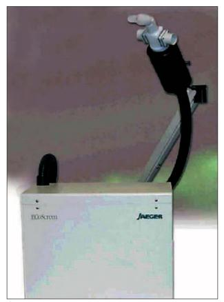
Figure 1. EcoScreen system (mouthpiece, connector, and cooling unit in the upper part of the figure) (Jaeger, Hoechberg, Germany).
